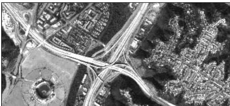
In this 2X (18 x 18 inch) enlargement of the same photograph, at a scale of 1:20,000, 1 inch on the photograph represents 1,666 feet on the ground.
