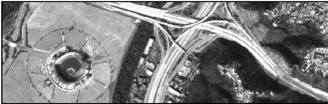
In this 4X (36 x 36 inch) enlargement of the same photograph, at a scale of 1:10,000, 1 inch on the photograph represents 833 feet on the ground.
